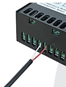
4. Disconnect the old flow switch connector and connect the new flow switch connector.
